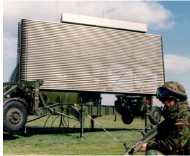
Figure 23. Commander AR327 - Type 101 air defense radar
