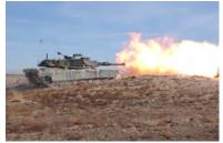
The M1A1 series main battle tank fires a 120mm smooth bore main gun and has three smaller caliber machine guns
