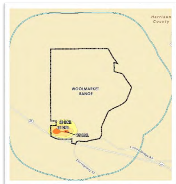
Figure 60 Above: Max Peak Noise from the JIEDDO course and the small arms range Below: DNL noise contours from the small arms range
